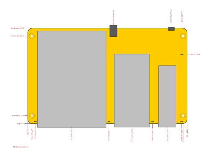
Overall board size: 120.0mm x 200.0mm Board thickness: 1.6mm.
