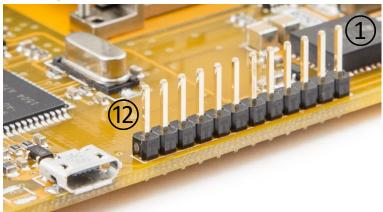
A 0.1" header is provided with access to the following connections:
