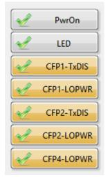
PwrOn controls the power to the CFPs. LED controls the LED to the right of the CFP4 transceiver. The other buttons control the status of various CFP hardware control lines.
