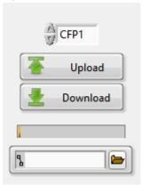
Use the Upload button to load a data file into the CFP. A dialog box will open, where the file to be uploaded is specified.
